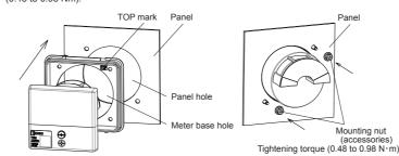
Make sure that the waterproof packing is properly installed inside the meter cover, and then insert the meter cover into the meter base.
